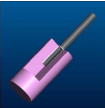
*A ceramic grinding wheel and a steel shaft are joined by a thin film of zinc alloy. A small amount of the molten alloy seeps into the stone and shrinks onto the shaft as it cools, securely bonding the components. The joining operation is completed in milliseconds. Compared to similar joints done with epoxy, the zinc alloy bond eliminates curing time, and the assembly is concentric as cast.*
